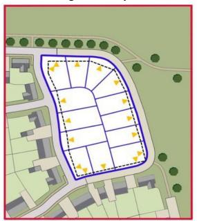
Plot Form - Plot form is defined by the width and depth of the plot. While this will likely vary from plot to plot, the size of plots within each area should be largely consistent as this will be informed by the masterplan vision, character area and the surrounding context including the proposed street type, landscaping and adjacent existing and proposed development. For example, more generous sized plots would be appropriate for development with a rural character and generous landscaping.
