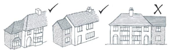
Figure x: The roof form of the side extension should reflect the roof form of the main house.
