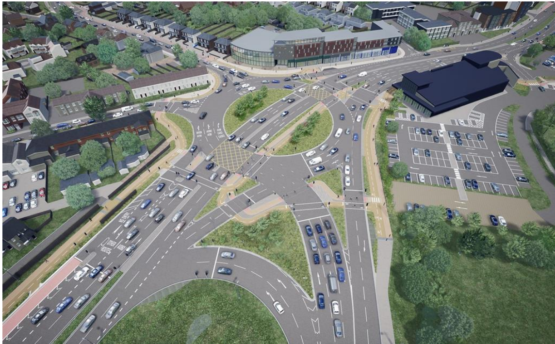
Figure 8-3: Concept image of the Army and Navy Roundabout proposed 'hamburger' layout.
