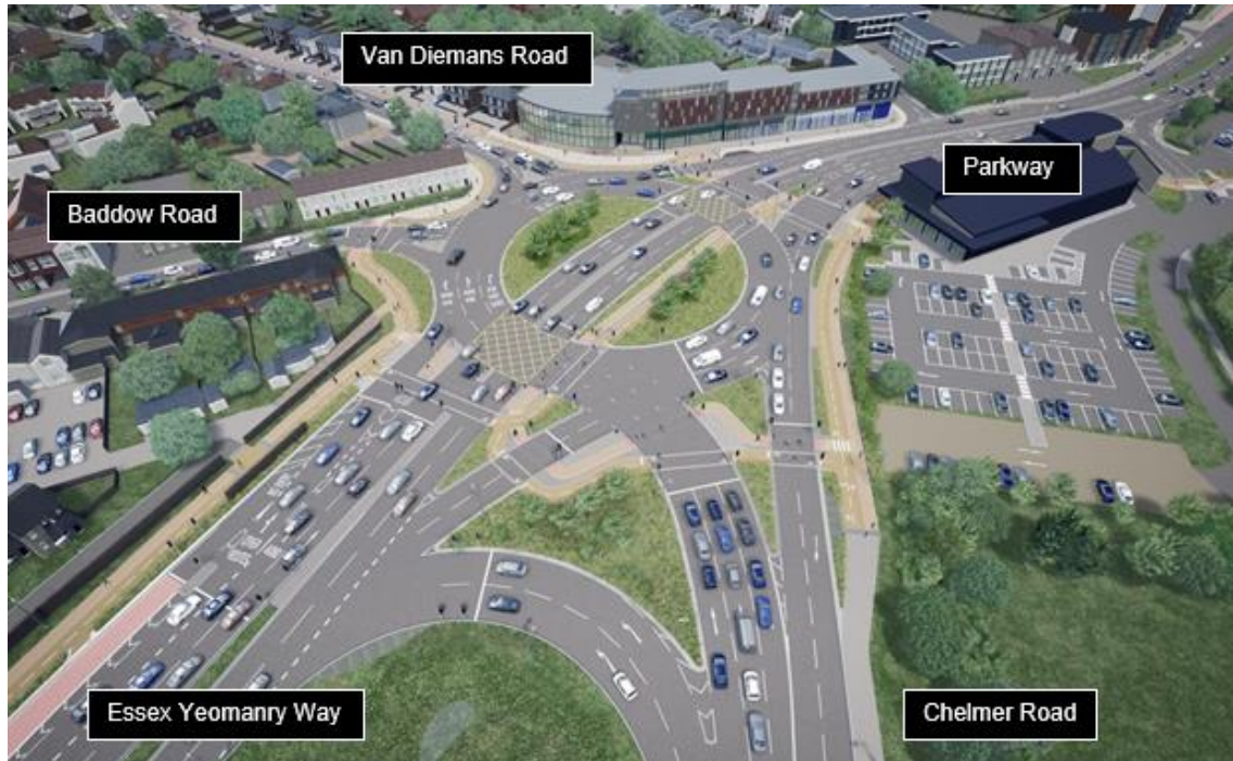
Figure 8-21: Concept image of the Army and Navy Roundabout proposed 'hamburger' layout.
