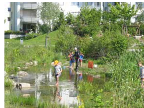
Shallow slopes, low water depth and stable edges minimise the need for fences and illustrate a designed approach to health and safety
