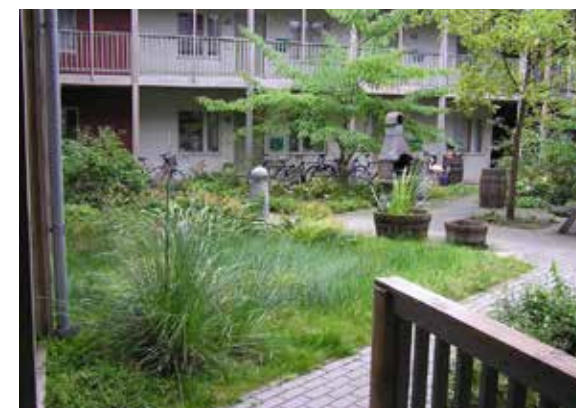
This rain garden controls surface water at source and provides habitat for wildlife.
