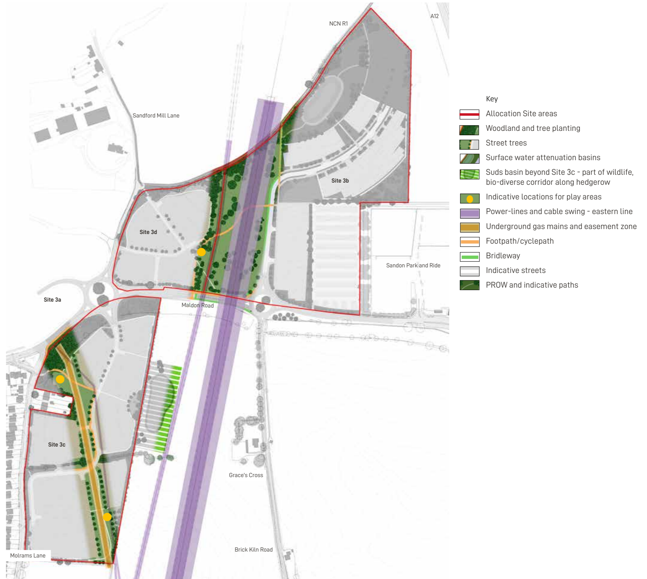
Gas Easement Overhead Line Safety Zones.
