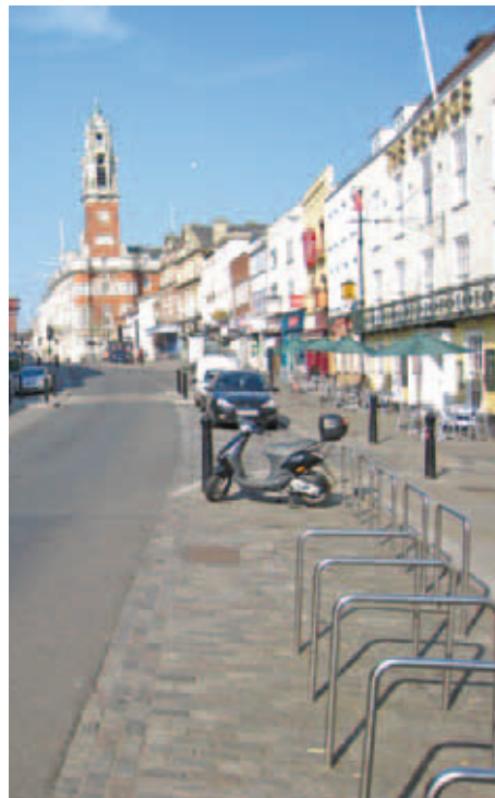
Short term PTW parking, note inappropriate cobbles and manhole cover within parking area
