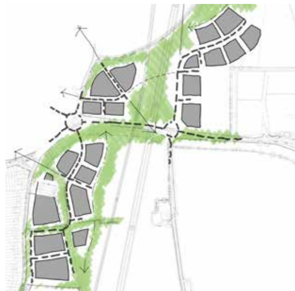
Testing the block structure/the landscape structure. Green corridors informed by existing landscape features including views, hedgerow, woodland and pill boxes structure the movement network and layout of blocks. Aligning key routes to corridors. Green corridors provide a succession of views into and through the development area providing for a highly legible layout
