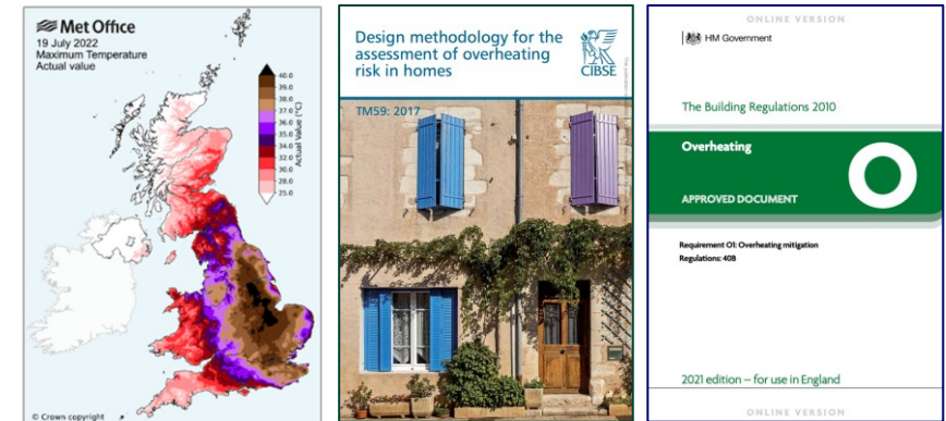
Figure 2: Severe heat waves such as occurred in 2022 are forecast to happen with increasing frequency, due to climate change. Building Regulations ( Part O ) requires mitigation to be incorporated into the design of new homes, based on the methodology described in CIBSE TM59 .
