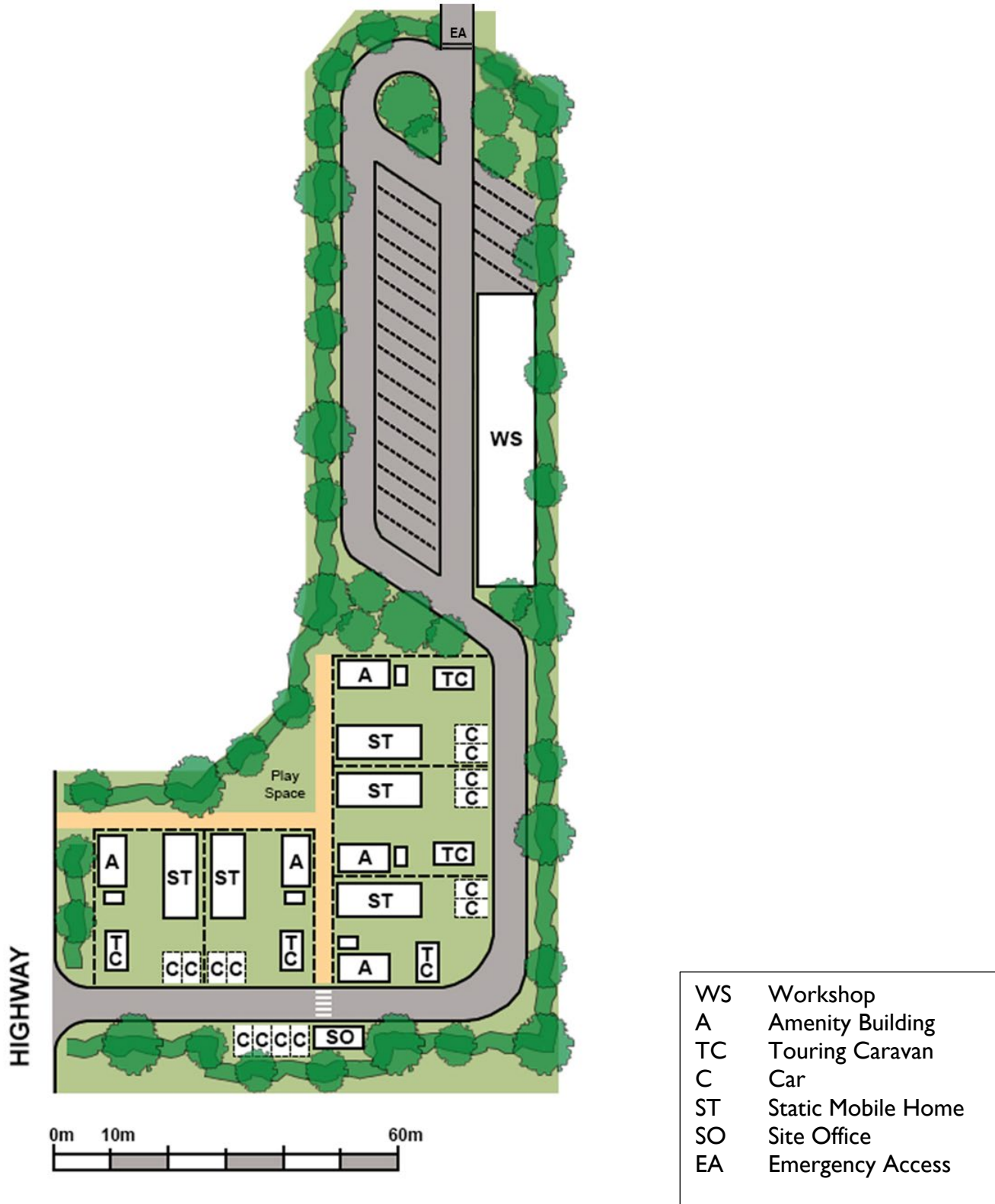
Figure 2: Indicative Travelling Showperson site example layout with shared provisions
