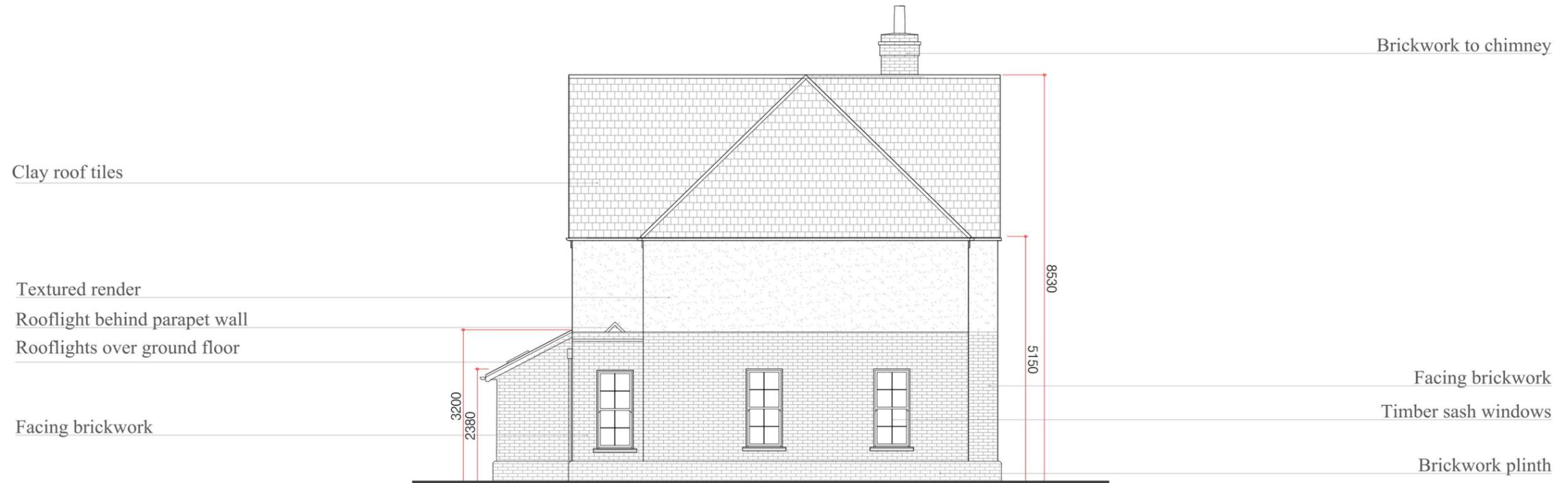
SOUTH ELEVATION DRAWING no. 2101. Scale 1:100@A3
