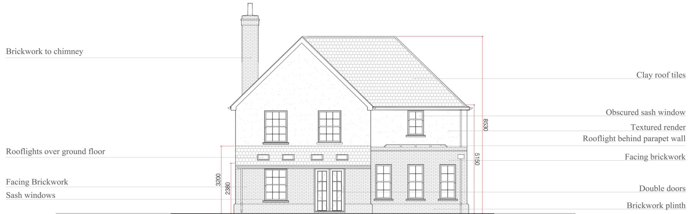
WEST ELEVATION DRAWING no. 2102. Scale 1:100@A3
