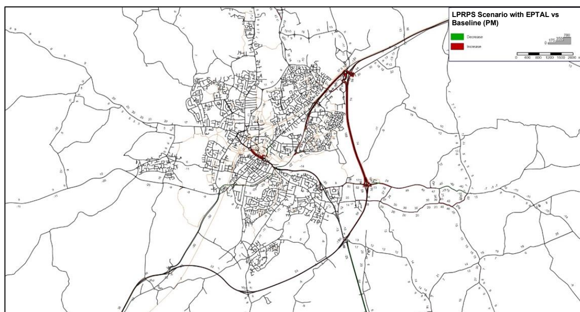
Figure 7-2: LPRPS Development with EPTAL vs Baseline - flow difference plot - 2041 PM Peak
