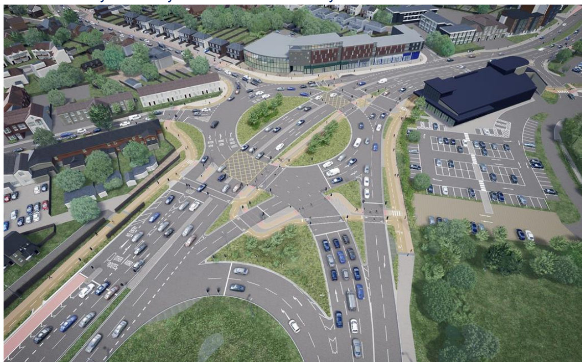
Figure 8-3: Concept image of the Army and Navy Roundabout proposed 'hamburger' layout.
