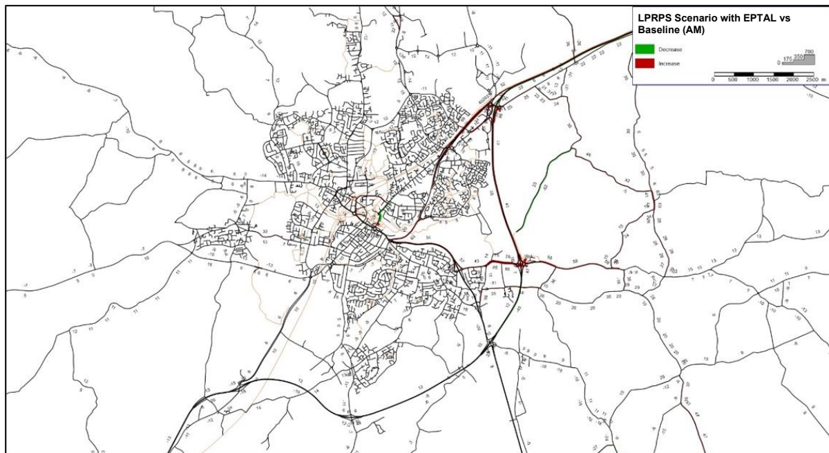
Figure 7-1: LPRPS Development with EPTAL vs Baseline - flow difference plot – 2041 AM Peak
