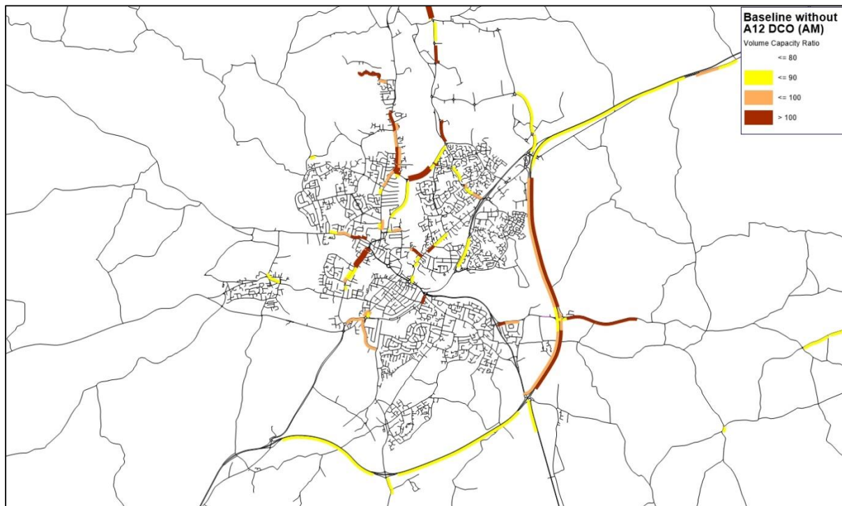
Figure 6-5: Volume/Capacity plot – Baseline without A12 DCO – 2041 AM Peak
