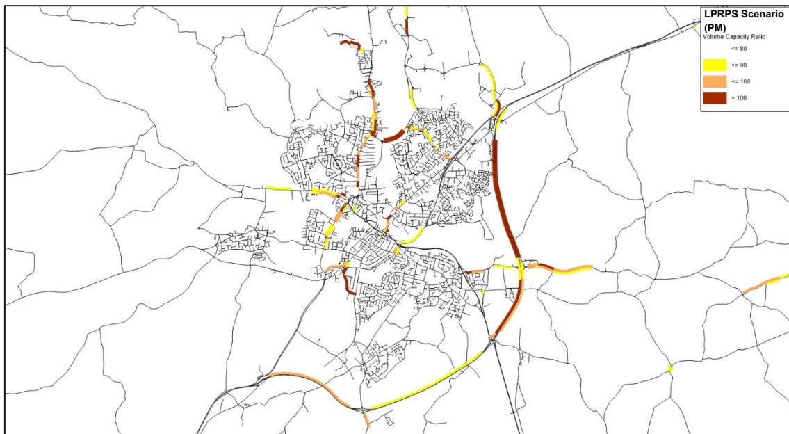
Figure 5-14: Volume/Capacity plot – LPRPS scenario – 2041 PM Peak
