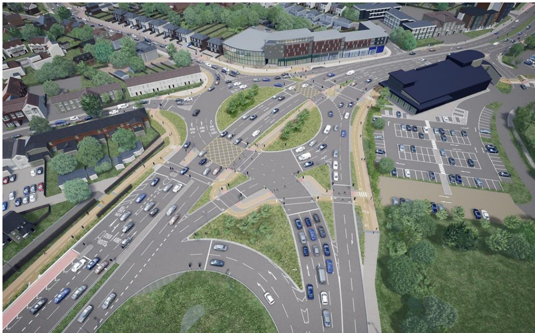
Figure 3-3: Concept image of the Army & Navy Roundabout proposed ‘hamburger’ layout 2
