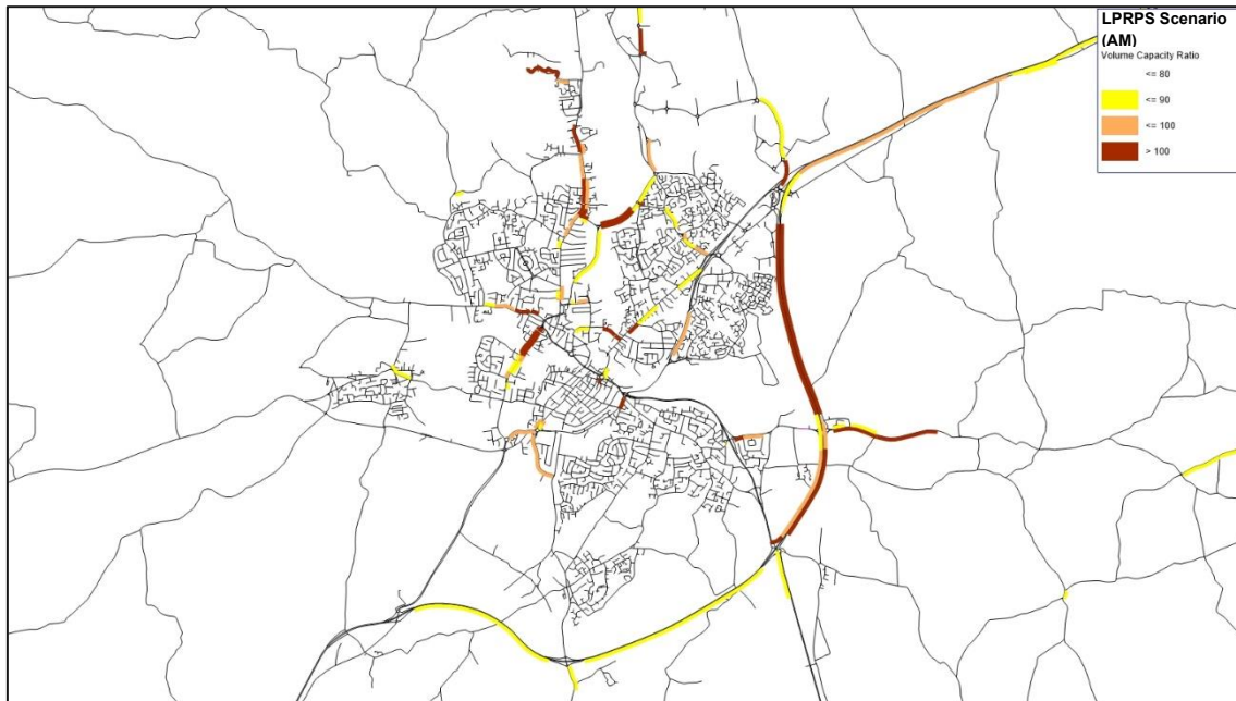
Figure 5-13: Volume/Capacity plot – LPRPS scenario – 2041 AM Peak
