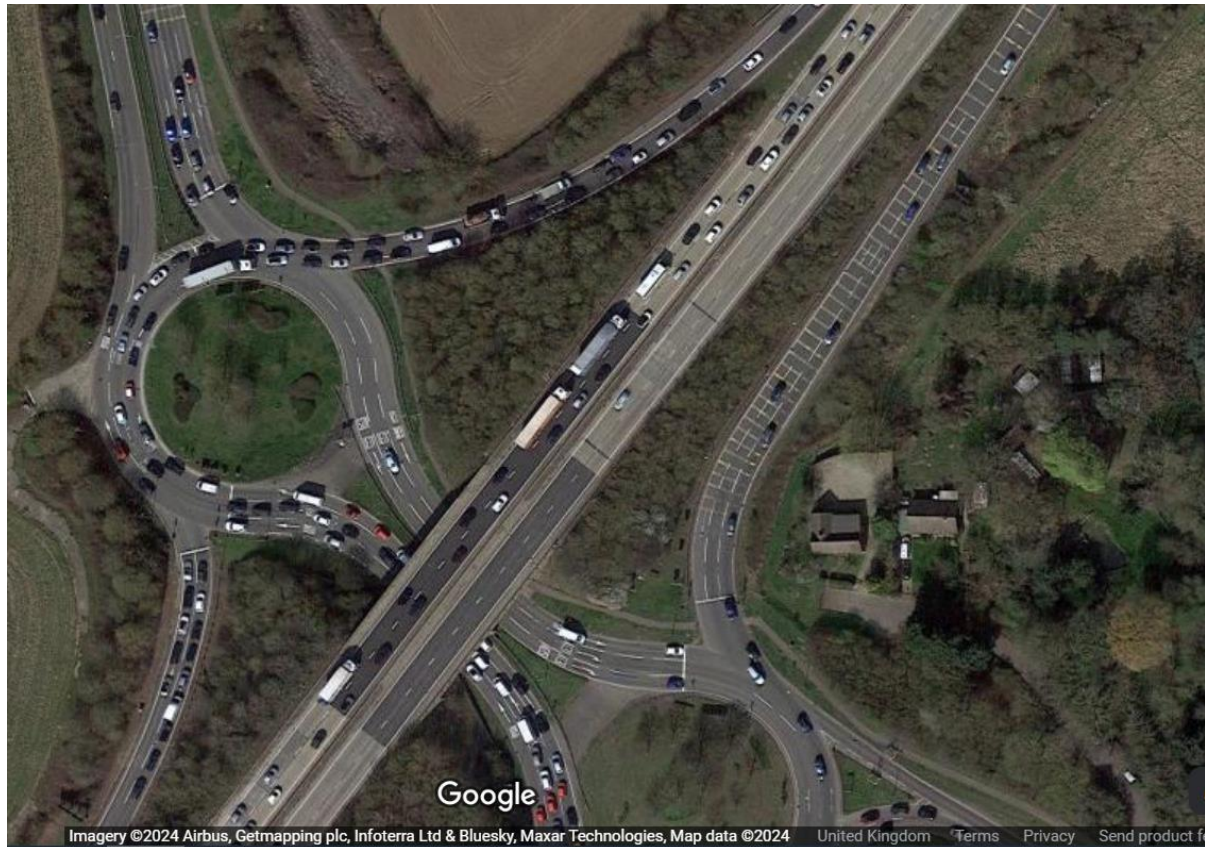
Figure 8-2: Google Maps screenshot of peak hour queuing on A12 northbound on-slip from J17 Howe Green
