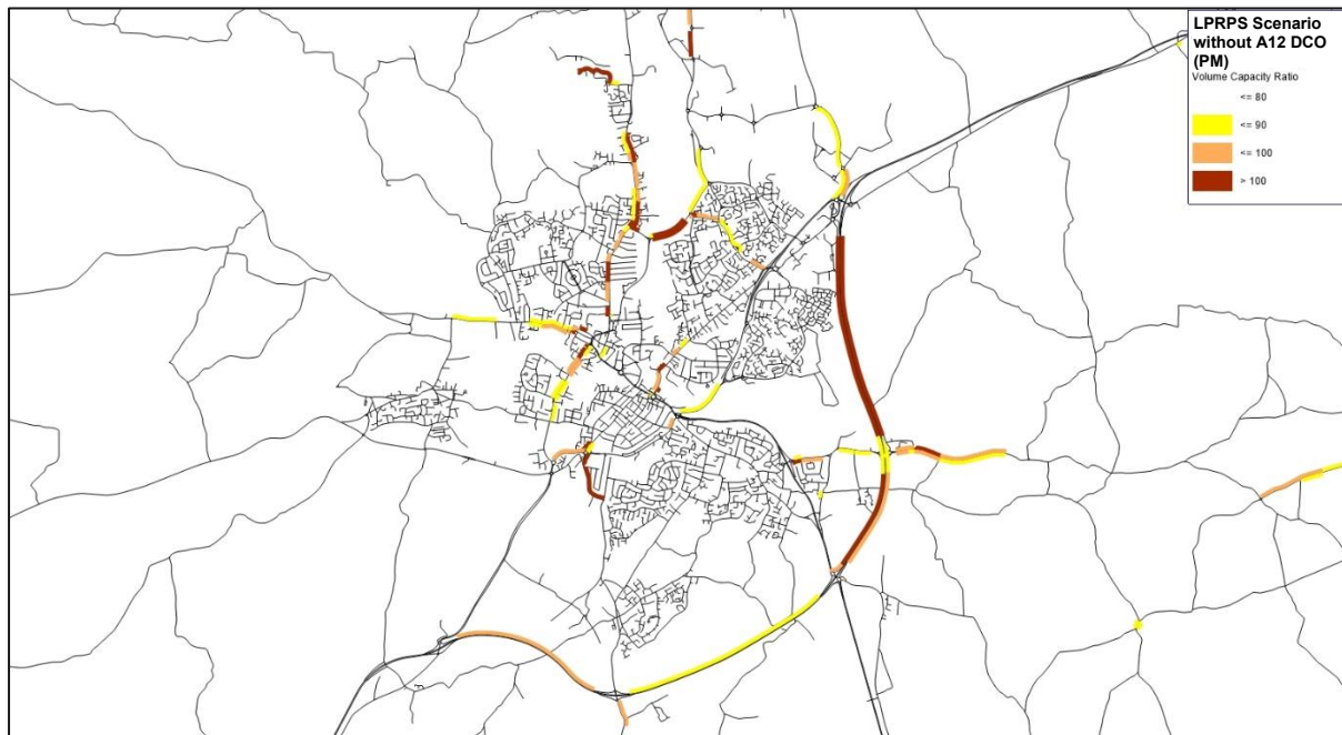
Figure 6-8: Volume/Capacity plot – LPRPS Development without A12 DCO – 2041 PM Peak
