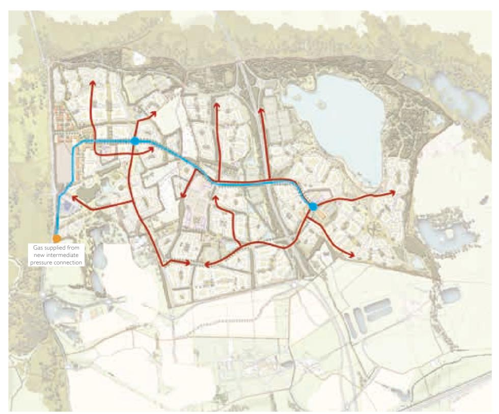
Cadent have confirmed we are able to connect to an existing Intermediate pressure main adjacent to the site with no reinforcement required. From this connection the pressure will be reduced to medium pressure via a pressure reduction installation for distribution through the site (shown in blue) The medium pressure network will supply 2no Pressure reduction installations on site for distribution to the development at Low pressure.
