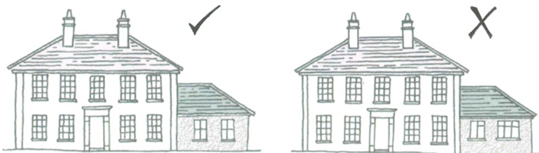
Figure x: The roof form of the side extension should reflect the roof form of the main house.
